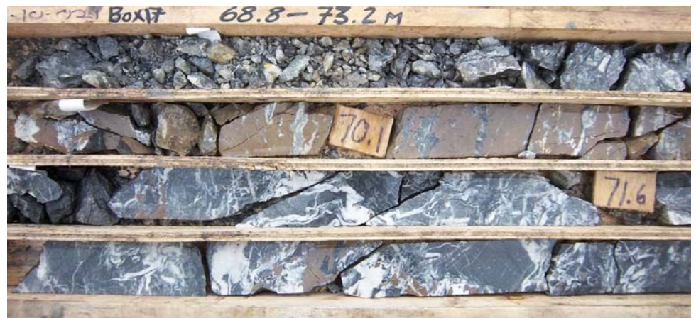
Figure 1. Massive, coarse grained zinc mineralisation intersected in DY10-021, extending mineralisation a further 100m to the west at the Darcy Zinc Deposit.
