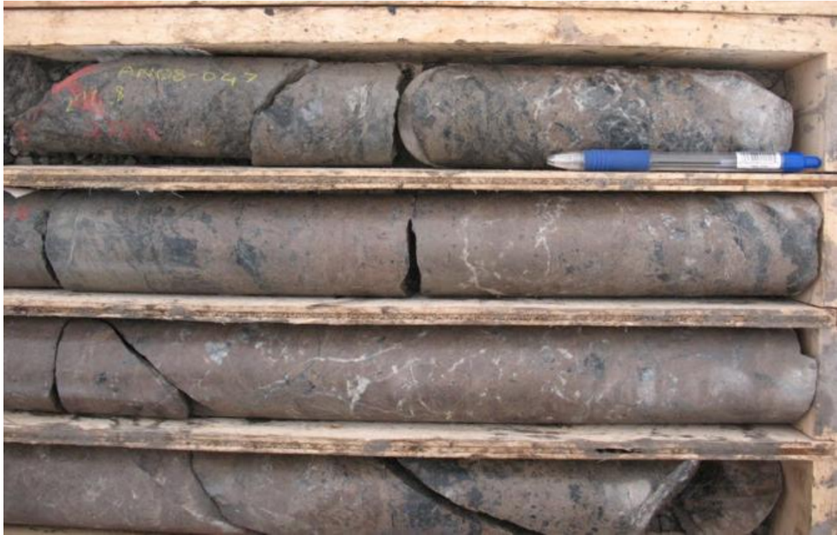
Figure 1: AN08-047: Massive sphalerite mineralization within 21.2m at 19.6% Zn from 272.8m.
