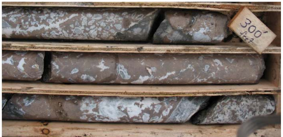
Massive, coarse grained zinc mineralisation intersected in DY-002, drilled recently at the Darcy Zone, Yukon Base Metal Project.
