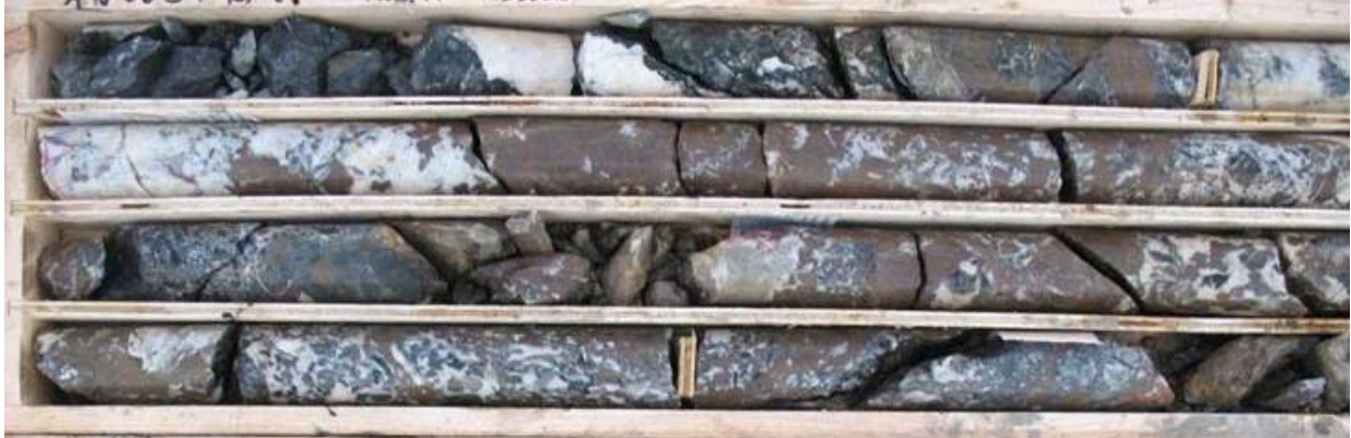
Figure 3. High grade zinc mineralisation (sphalerite) in diamond core from hole AN08-034
